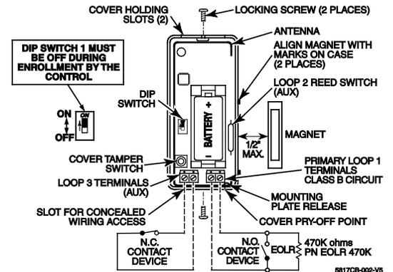
Figure 3. 5817CBXT Transmitter, Top Cover Removed
