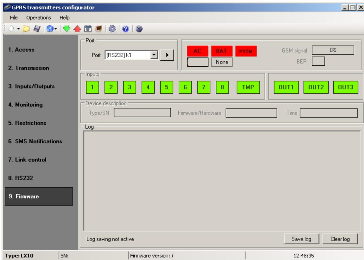
“Device Monitor” provides real-time information about device state. To use this function device must be connected to PC computer with LX-DATA cable (using DEBUG plug). Correct RS232 port must be chosen in “Port” field. “Device monitor” provides following information:
